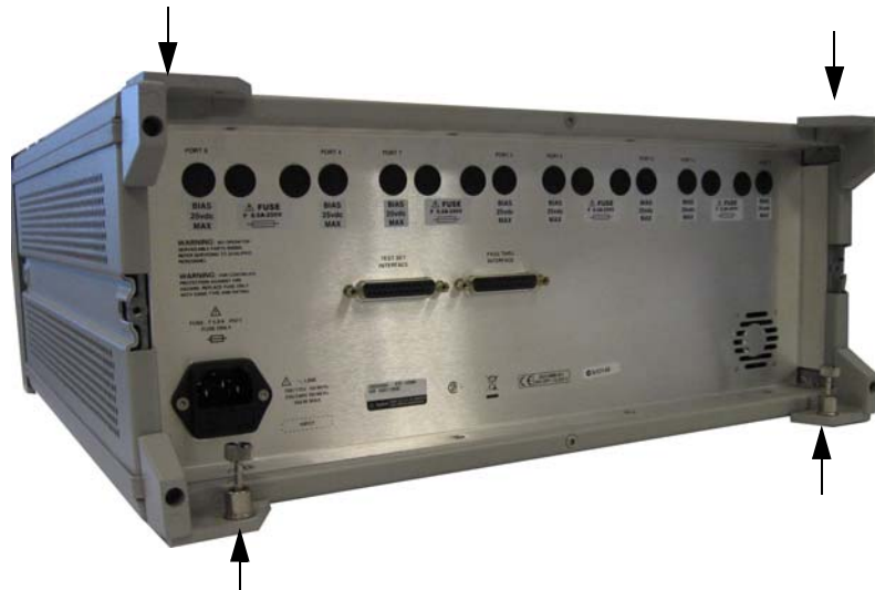
Figure 14 Installing Lock Feet
